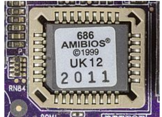
BIOS chip in a PLCC package
