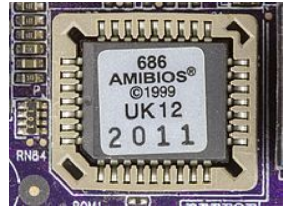
BIOS chip in a PLCC package
